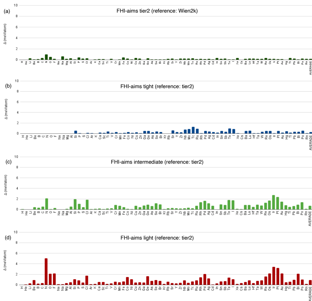
Figure 9.1: The \Delta gauge [42] between (a) WIEN2k and FHI-aims with really tight settings and tier2 basis functions (tier2), (b) FHI-aims tight and tier2 (c) FHI-aims intermediate and tier2, and (d) FHI-aims light and tier2.
